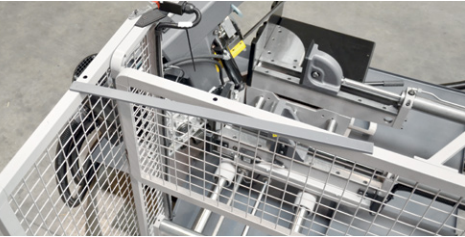
Workline automatic machines are enclosed with a safety grid. When performing mitre cuts, the rear cover shall be open, preventing the performance of the automatic cycle.
