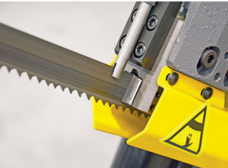
The band-saw blade guides of the Workline series are equipped with accurate grinded guidances from the hard metal. The haul-back blocks in front of the guides are lightening the band-saw blade and increasing accuracy.
