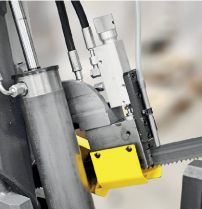
The automatic cutting pressure regulation automatically adapts the cutting feed and pressure to the material. The result is higher cutting output and longer service life.
