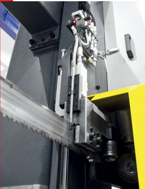
Hard-metal guidance of the saw band ensure high cutting accuracy..
