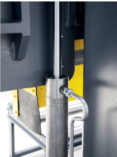
Hard-metal guidance of the saw band ensure high cutting accuracy..
