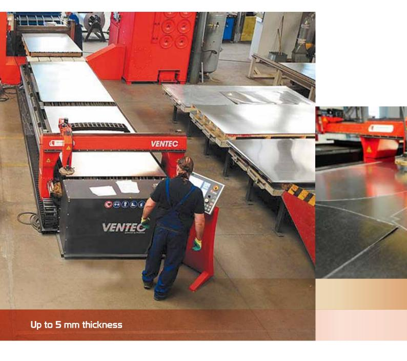
Ventec is a complete cutting solution for production of ductwork, that is applied in the heating and ventilation industry (HVAC).
