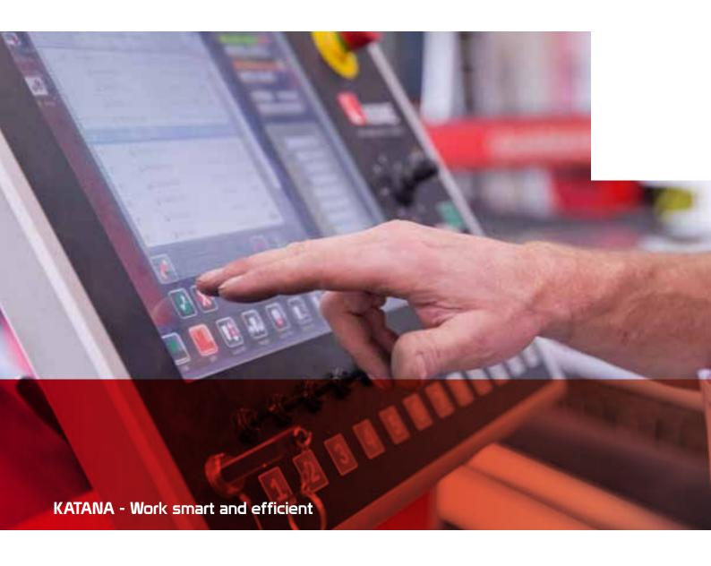
KATANA is the KOIKE global control for cutting machines and is equipped with a touch panel for superb multi-tasking efficiency while featuring an intuitive user interface.
