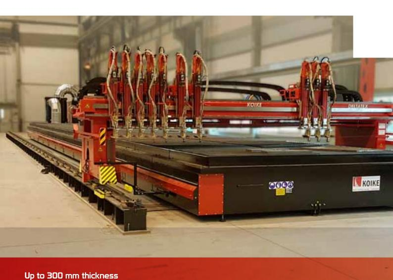
Deltatex is a robust gantry machine developed to meet the highest demands on precision, ease of operation and performance. Deltatex is engineered to work in the toughest production environments and suitable for multi-shift operation.
