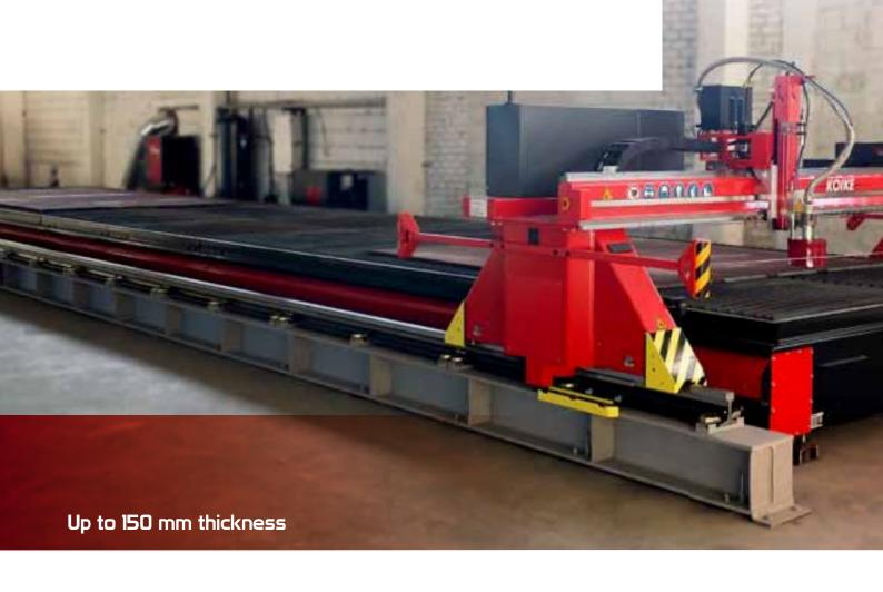
Deltatec is a highly accurate gantry machine developed for precision thermal cutting in heavy duty production environments. The machine is built with the use of the latest process control technology combined with excellent mechanics resulting in a rigid, dynamic machine.
