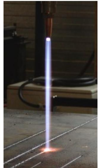
*Strong cutting oxygen stream from a Divergent nozzle: Photo taken from Koike in-house performance test. Nozzle tip at 275mm above the plate, nozzle 106-D7#0.*
