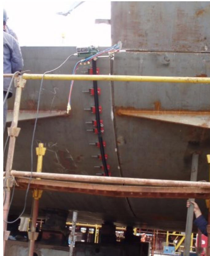
*Welding preparation performed with 2D rail*
