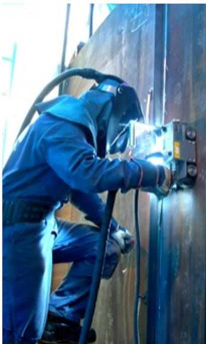
Vertical up butt welding using guide rail
