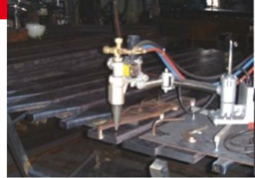
IK-82 M300 being used for profile cutting
